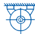
IM B8 (IM 1 071) Shaft horizontal Feet viewed on DE upward Mounting to ceiling
