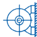
IM B7 (IM 1 061) Shaft horizontal Feet viewed on DE to the right Mounting to wall
