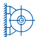
IM B6 (IM 1 051) Shaft horizontal Feet viewed on DE to the left Mounting to wall
