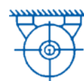
IM B8 (IM 1 071) Shaft horizontal Feet viewed on DE upward Mounting to ceiling
