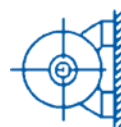
IM B7 (IM 1 061) Shaft horizontal Feet viewed on DE to the right Mounting to wall
